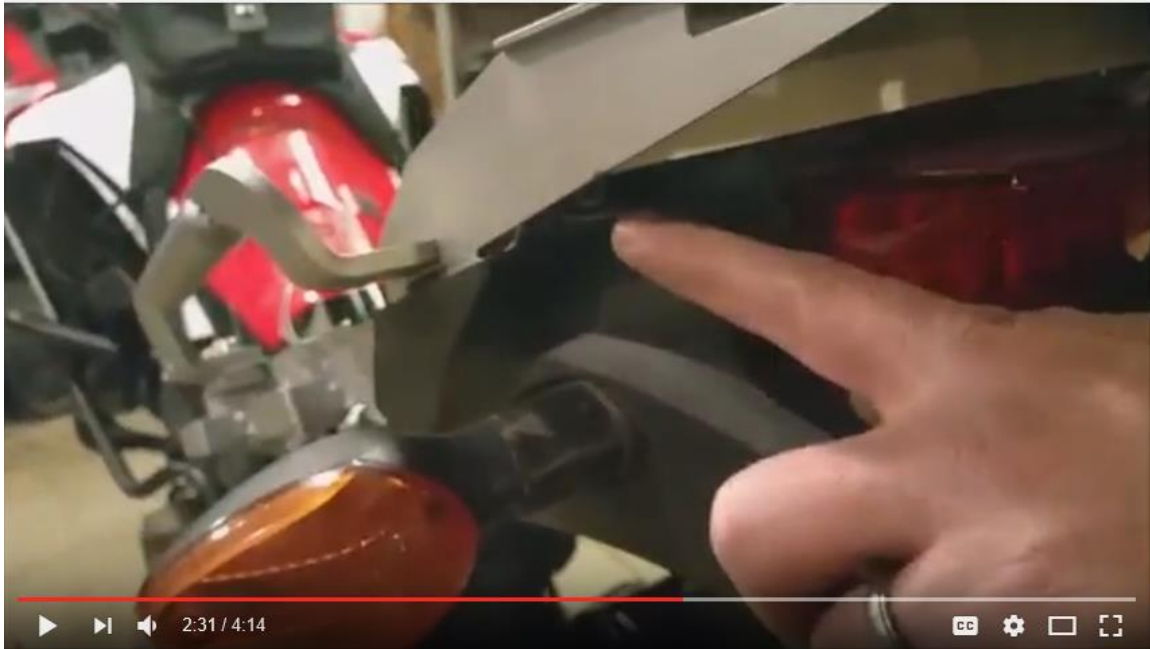
Install two OEM M6 socket head shoulder screws to secure the taillight assembly.
