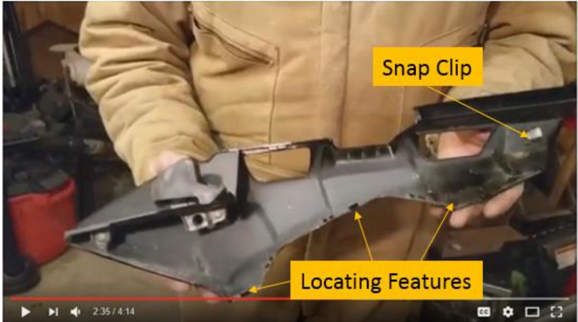
Fascia locating features engage fender; snap clip inserts into slot on ATO rack.
