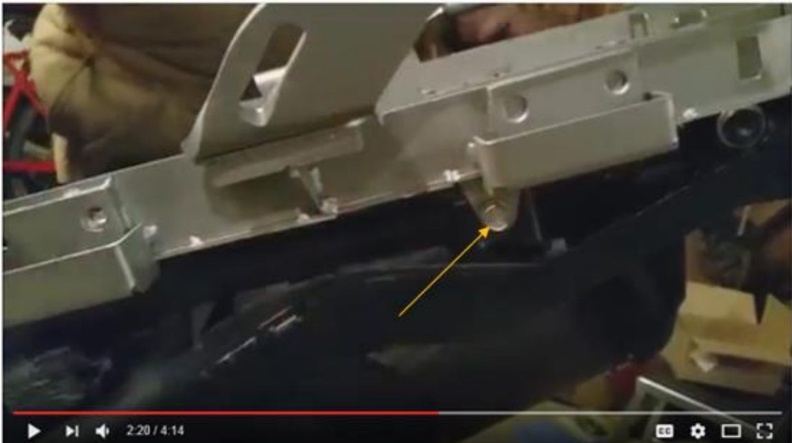
Install two OEM M6 hex bolts, one on each side.
