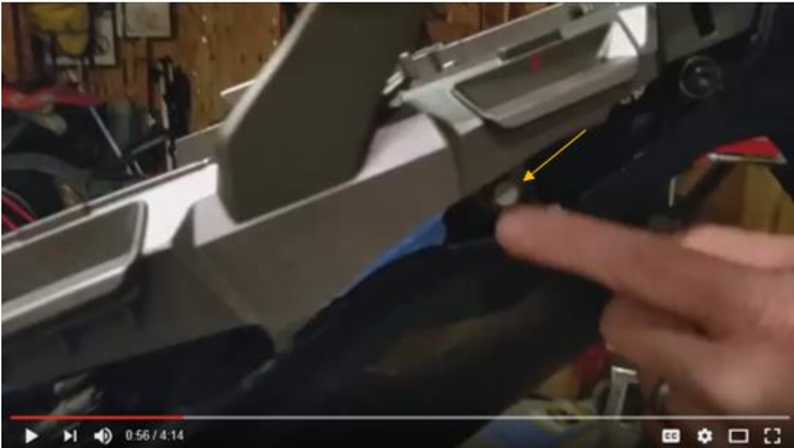
Remove two M6 hex bolts, one on each side.
