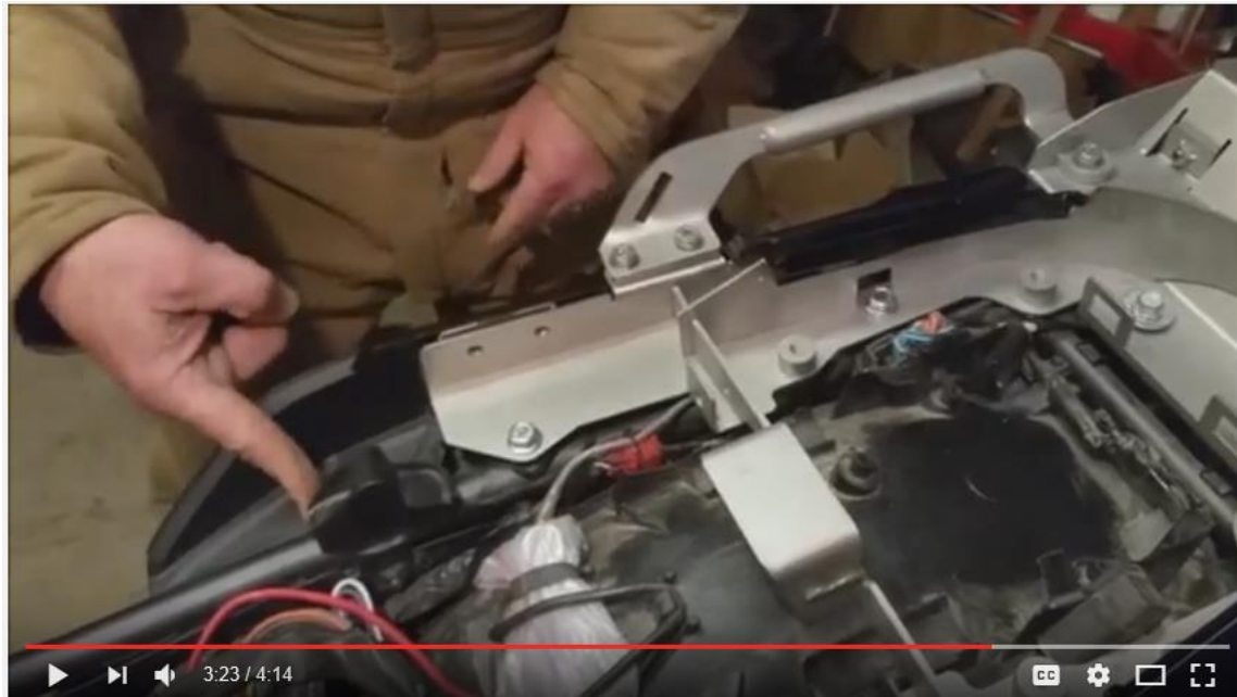
Engage snap clip into mating slot in rack and install OEM bolt securing front of fascia.
