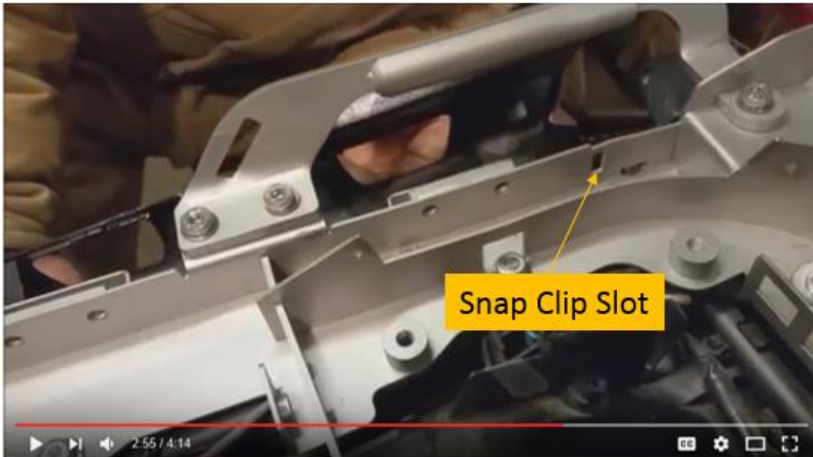
Engage fascia locating features with mating surfaces in fender.
